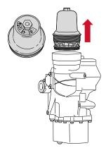
3. Turn the screw cap clockwise to unlock the centrifuge base.
