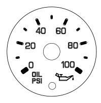
It is important to maintain oil pressure within acceptable limits. If oil pressure drops below the minimum psi a red warning lamp on the oil pressure gauge and the Stop Engine Lamp will come ON.
