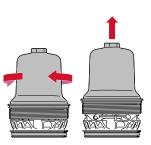
Press the clips (1) and dismount the centrifugal oil filter element from the centrifuge base.
