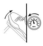
To reduce vehicle speed, put the engine brake or exhaust brake ON/OFF switch in the "ON" position. Remove your foot from the accelerator pedal and clutch pedal. The engine brake or exhaust brake will immediately begin to operate, slowing the vehicle.
