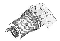
Clean the fuel bowls and filter housing of any sediment or debris. Look directly down into the filter housings from above for any signs of dirt or debris. If necessary, use a light. Remove any debris that can be seen
