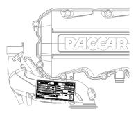
The engine label provides many details regarding the engine. Some facts that are found on the EPA label include the following:
