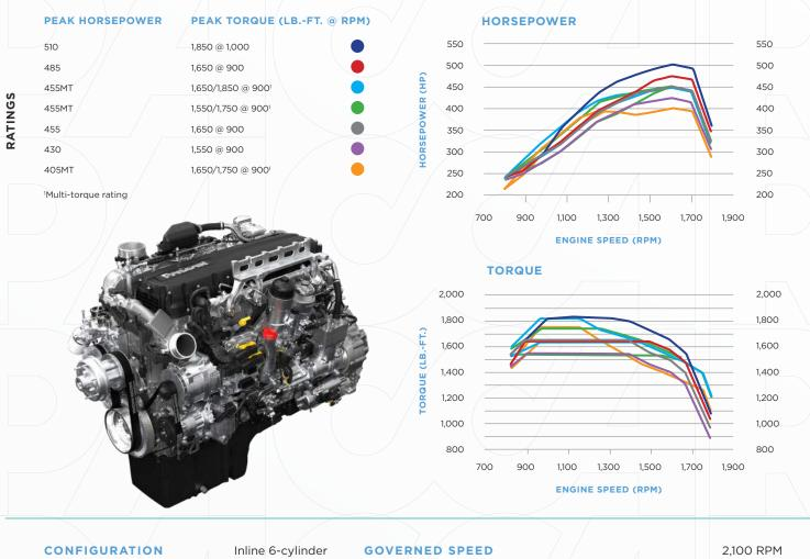
SPECIFICATIONS BORE X STROKE (MM) 130x162 **BASE WARRANTY<sup>2</sup>** 2 YRS./250K MI./400K KM. DISPLACEMENT 12.9 L. MAJOR COMPONENTS WARRANTY 5 YRS./500K MI./800K KM. **DRY WEIGHT** 2,500 LBS. CERTIFICATION EPA 2024 **OIL SYSTEM CAPACITY** 42 U.S. QTS. MAXIMUM OPERATING WEIGHT 140,000 LBS. HORSEPOWER 405-510 HP 1,550-1,850 LB.-FT. PEAK TORQUE <sup>2</sup>Extended protection plans available
